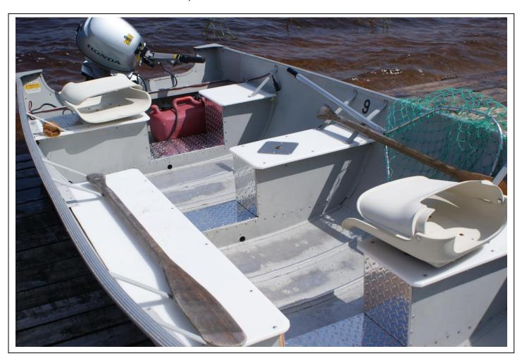
Ryan and Bill converted 7 of the boats in 2017 so the race was on to get the final 6 done this season. Everyone loves the modified boats at Goose Lake. They feature 9.9 hp Honda 4 stroke motors with electric start, 12-volt outlets for fish locators,
